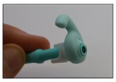
Adjust length of earpiece by gripping rigid Handle (4) with thumb and finger, and push or pull the earpiece in and out with the other hand whilst viewing the live camera feed.
