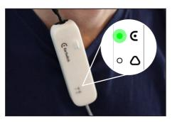
If the earpiece falls out during use, an amber *Advisory* LED will appear on the lapel clip (2) and Control Box (1). If this LED appears, firstly check with the user they are okay, then reposition the earpiece and press + or - button to reset the device
